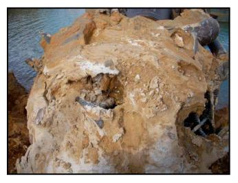
A typical bladed style cutter basket with sizing bars completely choked with clay and near-size material.
