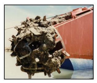
A sand & gravel screening style cutter basket plugged with clay and near-size material.
