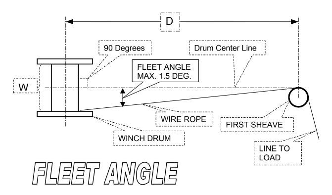
The fleet angle depends on two factors as shown on the above sketch—the width of the winch drum (W) and the distance between the drum and the first sheave (D). The chart below can be used as a guide to determine the minimum distance (D) that corresponds to a fleet angle that will not exceed 1.5 degrees for various winch drums (W). Distance (D) is a minimum. There is no limit to the maximum distance (D).
