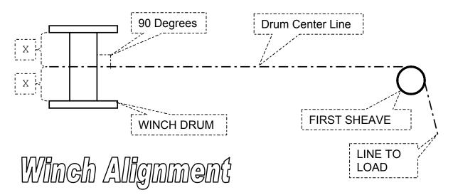
If the cable piles up on one end of the drum it is misaligned. If cable piles up in the middle of the drum it is likely that the fleet angle requirement has been abused.
