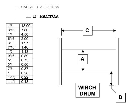
Use the formula: Drum Capacity in feet = (D + A) x D x C x K Factor for cable size
