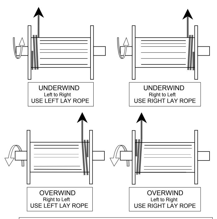
If a winch is aligned and cable still keeps piling up on one part of the drum the problem could be that the wrong cable is being used. *Willard Says.....* Wire Rope tells how to identify different styles of wire rope. The above sketches show various winch arrangements with the recommended style of wire rope for each.
